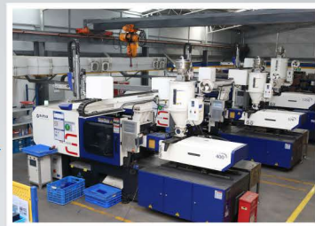
Injection Molding of Plastic Component (Injection Molding Machine | Material: PA66 + POM)
