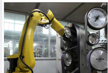
Polishing of Zinc Alloy Product (Robotic Polishing)
