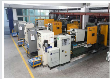
Die Casting of Zinc Alloy Product (Hot Chamber Die Casting Machine | Material: ZnAl4)
