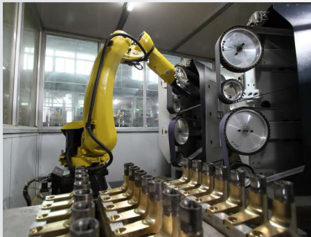
Polishing of Zinc Alloy Product (Robotic Polishing)
