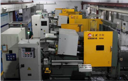
Die Casting of Zinc Alloy Product (Hot Chamber Die Casting Machine | Material: ZnAl4)
