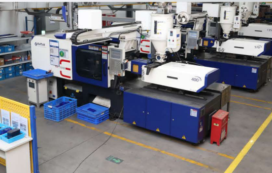
Injection Molding of Plastic Component(Injection Molding Machine | Material: PA66 + POM)
