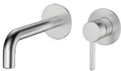
BW1912A Single lever concealed basin mixer Material: 304 Stainless Steel Panel: 304 Stainless Steel Cartridge: 35mm Smart box
